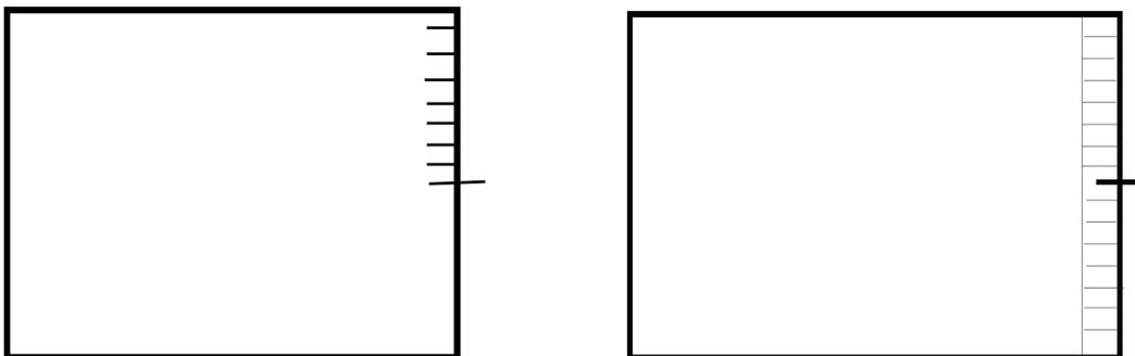
8. Measure the distance from the long wall to the starting line (center point) of the end wall (**A**). Measure and mark an equal distance from the long wall on the opposite end wall (**B**). Then chalk a line the length of the room between the starting points of the two end walls (**Z**). This line is parallel to the long wall.
