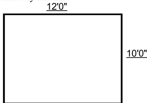
4. Check the exact dimension of the longest wall; determine the center point of the longest wall by dividing length by two, and mark the center point. Check your measurement again. Given the dimensions of the room above, and assuming that the walls are perfectly square, the wall will divide into two 6' 0" sections...
