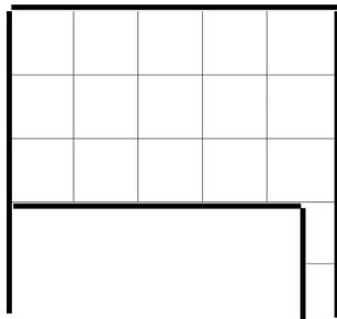
Step 3: Convert the dimension from (c) to (d) into inches:  $5'10'' = 70''$ . The  $2\frac{1}{2}''$  cut at the door frame must be subtracted from this dimension, leaving  $67\frac{1}{2}''$  as the dimension remaining to finish the wall.
